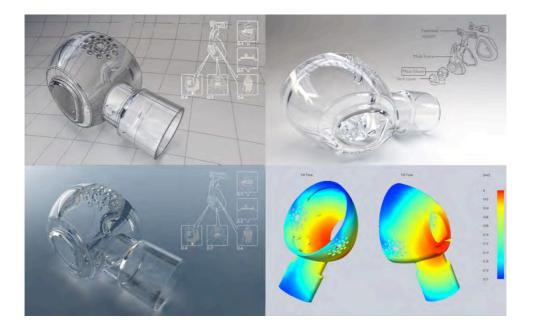
Figure 2. Nasal Mask Elbow Component, 2008. NURBS surface model, HDRI (High Dynamic Range Rendering) with caustics and design verification. Paul Kouppas
